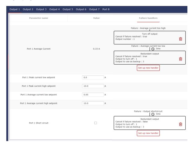
The failure handlers have been set. When the MaNima Pollux measures a shortcircuit it will disable the output (1) and activate the secondary output (3).
