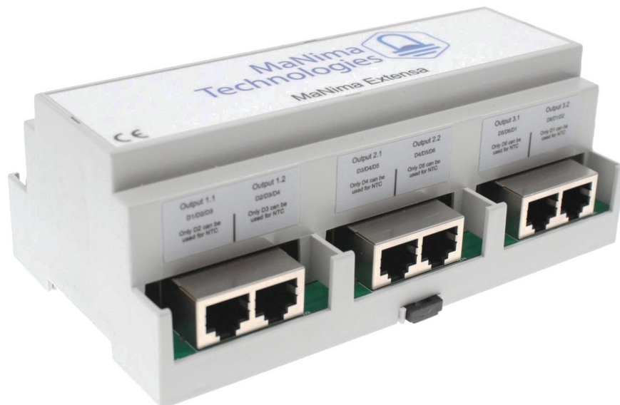
Figure 2 — Extensa, bottom face: the six RJ45 outputs. Each is labelled with the three datalines it carries and the one of those three that can carry an NTC signal.
